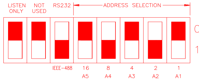
Figure 8-3: GPIB Address Selection Switch
